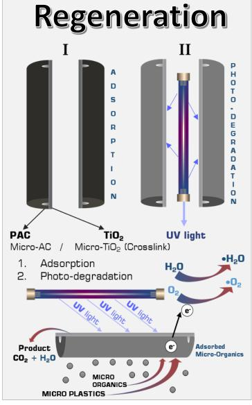
**50 to 200 times greater** than those of conventional carbon blocks. In addition, the cartridge can be regenerated continuously for very long time using a **UV lamp** (Light) in carbon blocks with no loss in performance. Finally, the **Titansorb-P** outperformed a leading **Activated Carbon block** for rapid, flow – through water treatment.
