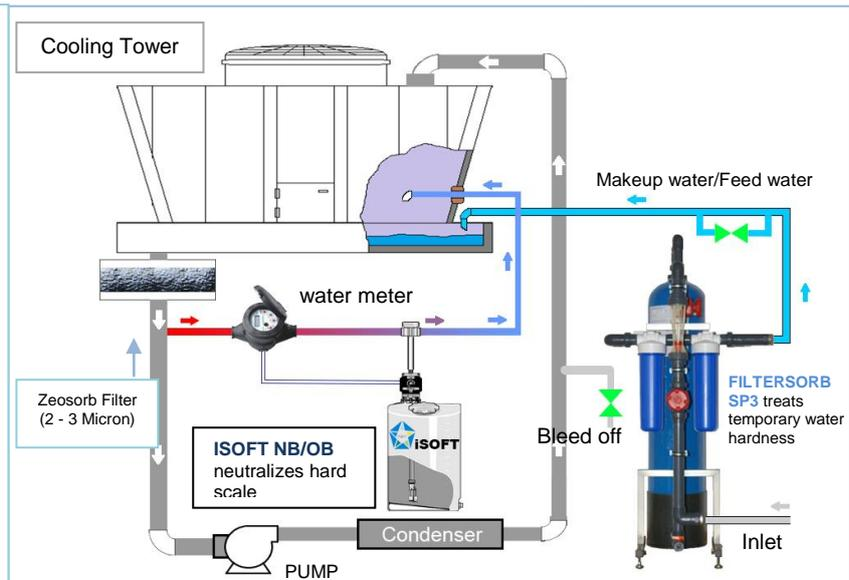
*Typical Cooling loop with complete Scale Prevention Solution*
