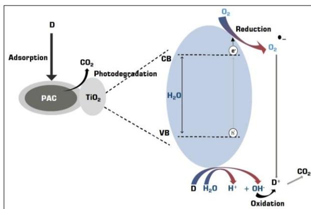
**Photodegradation** of organics and **adsorption** of inorganics to achieve **Adsorption-Desorption** equilibrium using powder activated carbon as **Catalyst** support the increase of **Photodegradation** rate by progressively allowing an increased quality of substrate to come in contact with **Titansorb** through means of **adsorption** and giving a complete photodegradation process.
