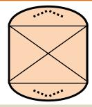
Simple reaction tank should be chosen to provide a internal contact time of 3 to 5 minutes
