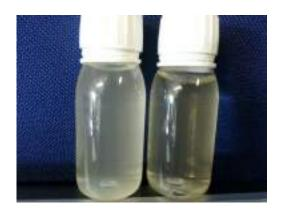
This shows that the filter is still working (clear water on RH side) at stopping scale build up after extensive use on water @ 550ppm.
