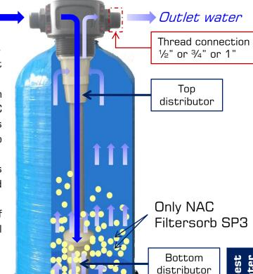
SPECIAL System removes lead (Pb) from Drinking Water
