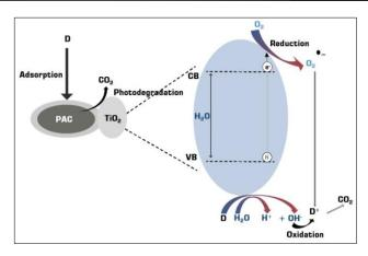
Photodegradation of organics and adsorption of inorganics to achieve Adsorption-Desorption equilibrium using powder activated carbon as <u>Catalyst</u> support the increase of Photodegradation rate by progressively allowing an increased quality of substrate to come in contact with **Titansorb** through means of **adsorption** and giving a complete photodegradation process.
