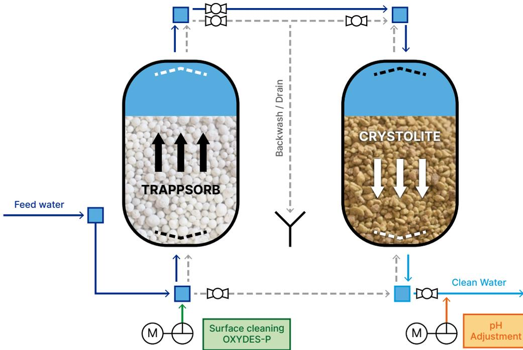
**OXYDES-P:** Oxidizing agent for surface cleaning. Depending on the water chemistry, it may be necessary to clean the surface of Trappsorb with OXYDES-P when the removal performance decreases.
