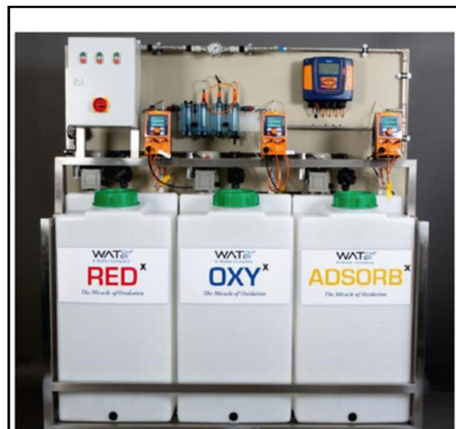
A real prototype of **REDOXY** Dosing system
